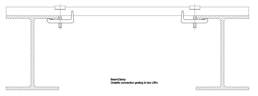
This block is a typical BeamClamp Gratefix application and is for illustration purposes only. The Gratefix is designed to allow open floor grating to be connected to the supporting steelwork without any penetration of the steelwork and no access to the underside is required. Please refer to web site or technical literature for full details of its use.
